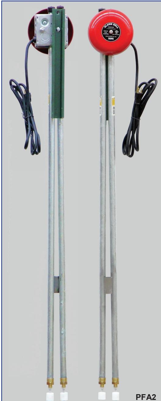
Our quality built 120VAC pit flood alarms designed for up to 4' deep pit and equipped with an 8' long power cord, 3-wire grounded plug, and 6" alarm bell. They are extremely adjustable, mounting to 8#, 12#, or 15# rails. One or two liquid level float switches installed on 4' galvanized rigid steel conduits (GRC). Mounting unistrut arm 1-5/8" x 13/16" x 14" and hardware included.
